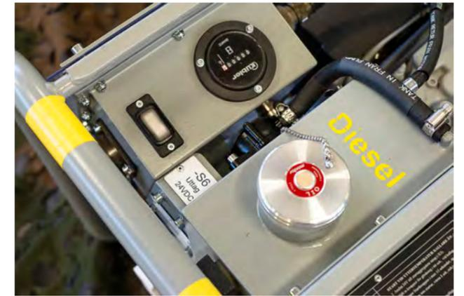
The GPU-Ts are heavy fuel compatible
