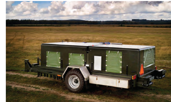
Trailer version with operating unit loaded. The boxes on the trailer houses all necessary accessories and tools.
