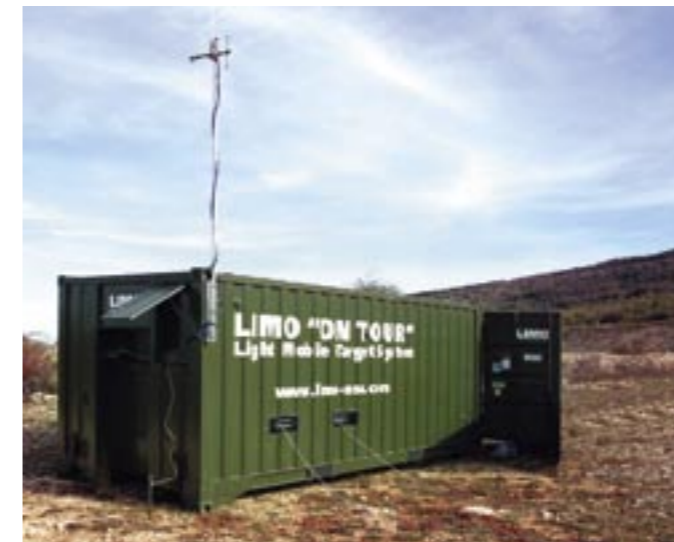
Container version with built in driving unit. In the standard 20 ft container there is also room for targets, remote control, tools and a small workshop.
