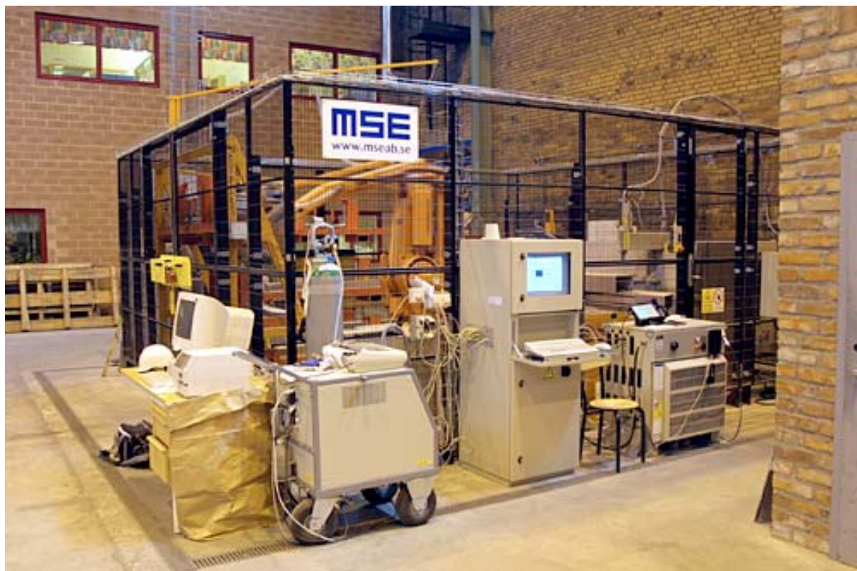
The analysis cell, where automated cutting and testing is carried out.
