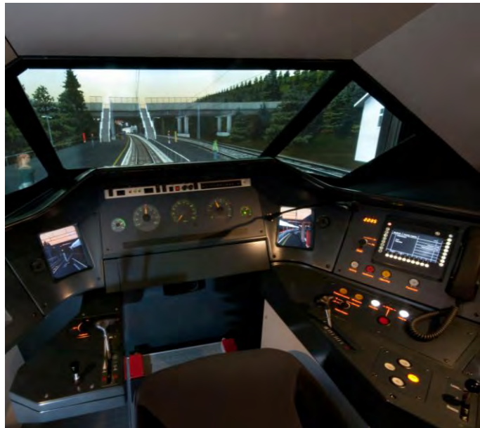
Interior of high fidelity train driving simulator
